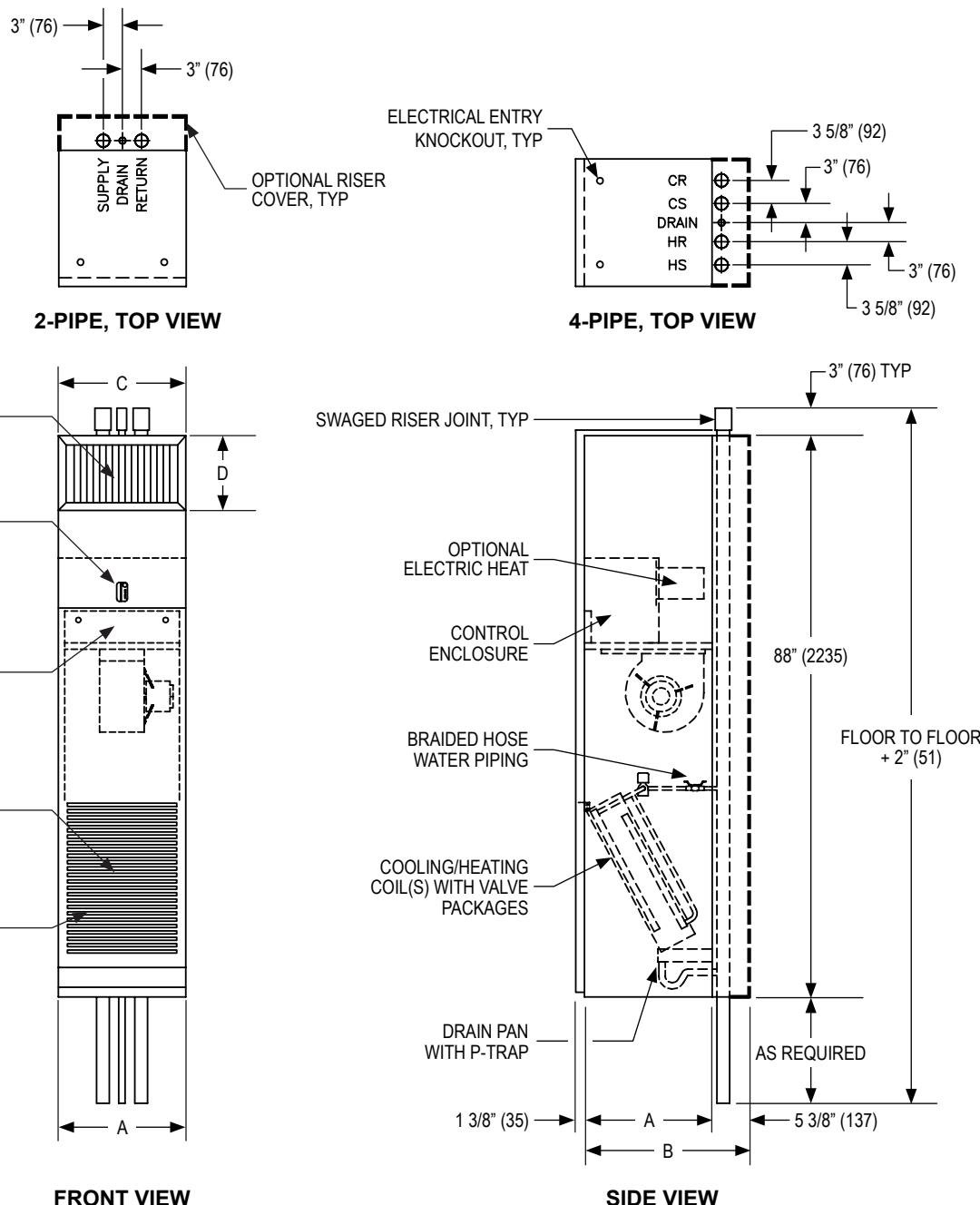
NOTE: Dimensions in parentheses are in millimeters (mm). See table below for dimensional references. Thermostat is shipped loose and may be unit surface mounted or remote wall mounted. All units are back riser, front single supply. Floor and ceiling trim furnished and installed by others.
